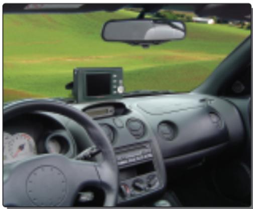
Position the unit where it is visible at a glance but will not obstruct the driver's view of the road or interfere with the use of vehicle instruments and controls.
