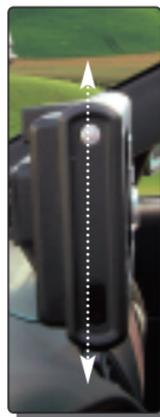
The unit should be as close to vertical as possible and not tilted front-to-back or side-to-side.
