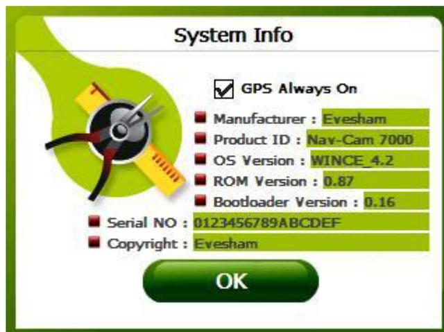
Here you can see your device's serial number, firmware version and GPS firmware version.
