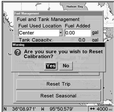
**Reset Calibration highlighted (left). Reset Calibration confirmation window (right). Reset Calibration will return the unit to the factory default calibration settings.**
