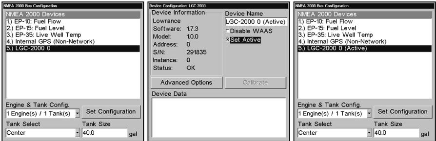
**LGC-2000 highlighted on Buss Setup menu (left). LGC-2000 Device Configuration menu with the Set Active checkbox selected (center). LGC-2000 is now listed as Active on the Buss Setup menu (right).**
