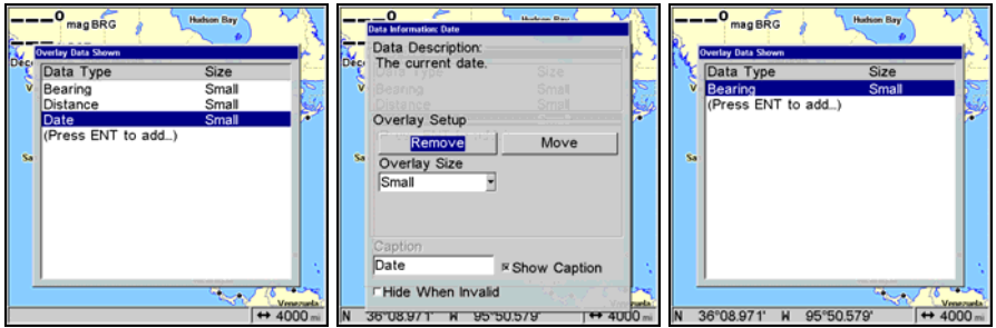
Overlay Data Shown menu with Date selected (left). Remove highlighted on Data Information menu (center). Date has been removed from the Overlay Data Shown menu (right).
