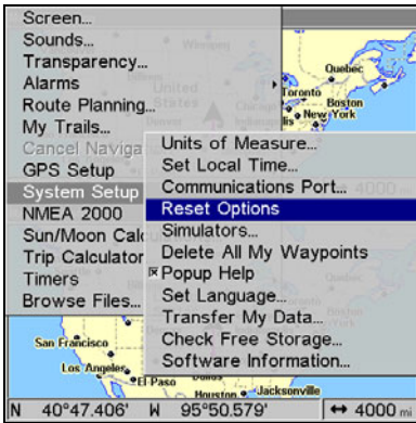
Reset Options highlighted on the System Setup menu (left). Reset Options confirmation message (right).
