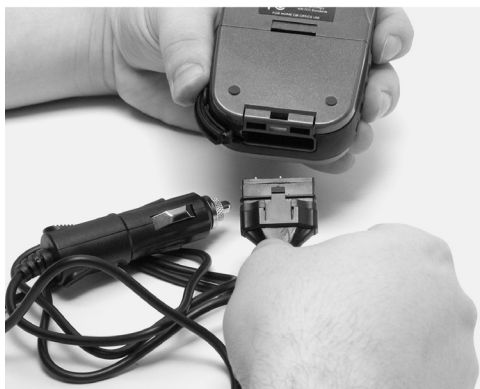
Attach external power cable to iFINDER.
