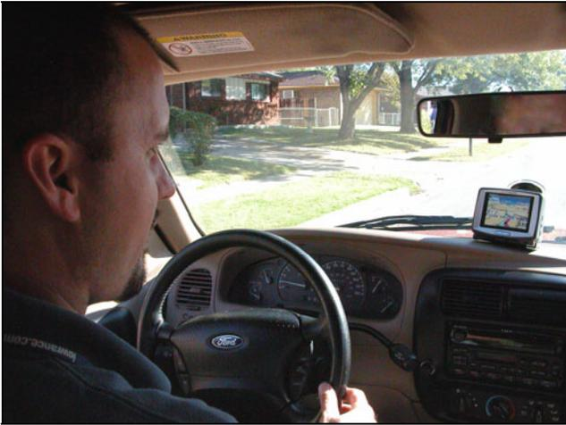
**iWAY™ 250c centered on a dashboard. This photo was taken at passenger eye level. Notice how the unit was placed so that it does not obstruct the view of the road ahead through the windshield.**
