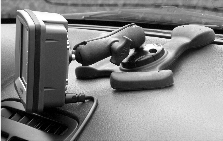
iWAY 500C mounted on dash with weighted base mount.
