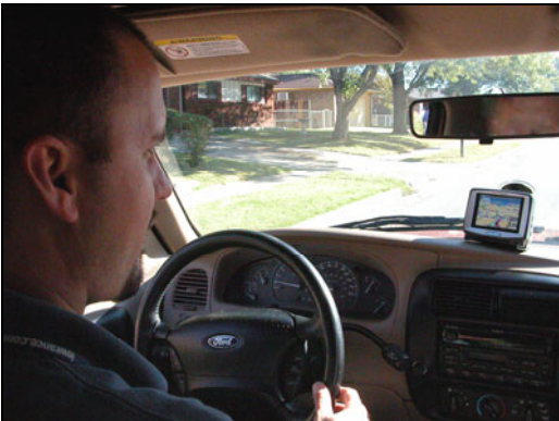
GPS unit centered on dashboard. This photo was taken at passenger eye level. Notice how the unit was placed so that it does not obstruct the view of the road ahead through the windshield.
