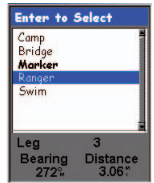
Route leg list with Ranger selected. Note that Marker is bold because it is the current active leg.
