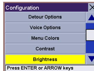
Select the left arrow to decrease the amount of brightness (make the display darker), or select the right arrow to increase the amount of brightness (make the display lighter). When you are finished, select **Save**.
