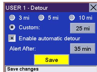
When you encounter traffic, and the set time has elapsed, the Detour icon will flash on the Map screen. Touch the icon on the screen to have the Magellan RoadMate calculate the detour. You can choose to ignore the Detour alert; and after one minute it will stop flashing until the set time has elapsed again when it will alert you once more.
