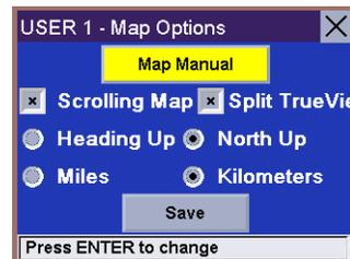
With **Scrolling** enabled, the vehicle position icon will always remain in the same position with the map scrolling, or moving as while the vehicle is in motion. With **Scrolling** disabled, the vehicle position icon will move forward slightly; then, the map will scroll down. Having Scrolling disabled allows for a faster display.
