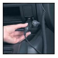
Rotate the antenna upward (see page 13 for proper antenna position).
