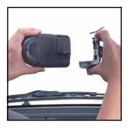
Slide the windshield mount onto the back of the car holder.
