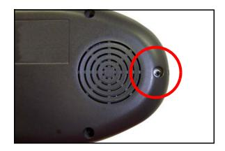
Remove the battery compartment cover.
